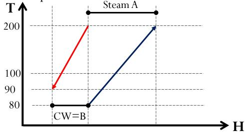
Alternatively, an improved scheme where the addition of a new 'Heat Exchanger— 3' recovers product heat (X) to preheat the feed. The steam and cooling water requirements get reduced by the same amount (X).
