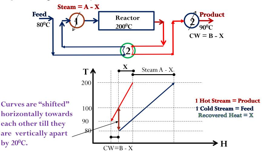
• The amount of heat recovered (X) depends on the 'minimum approach temperature' allowed for the new exchanger.
